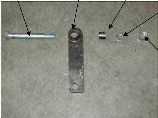
Rolling tongue Lever Arm Assembly – two sets required per assembly
